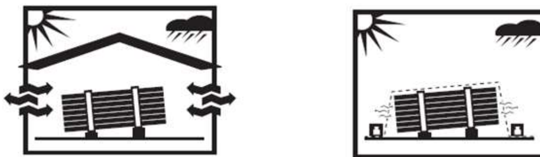
Figure 18 – Stockage des bacs Kalzip®
